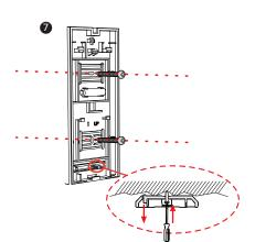
Note: When the wall surface is uneven, you can adjust the tamper screw.
