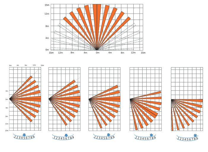
There are 5 scales in the vertical direction to adjust the detection distance. The default angle is A and the detection range is 15 m.
